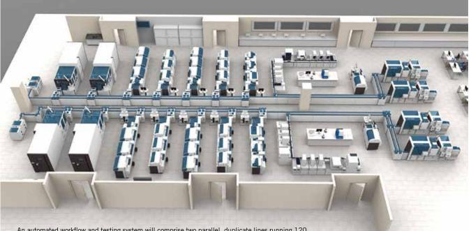
An automated workflow and testing system will comprise two parallel, duplicate lines running 120 linear feet, enabling Northwell Health to process up to 20 million tests annually, around the clock.
